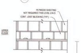
STUD SUPPORT FOR BEAM
