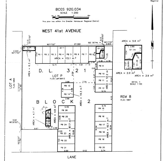
Bearings are Grid bearings and are derived from Plan LMP33612 All angles are 45 or 90 unless otherwise noted.
