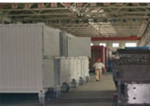
3rd primer coat, ready for paint
