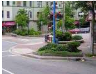
Lonsdale & 1st Street Intersection Example for Corner Bulges (Same as on the west side of the intersection)
